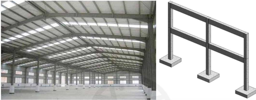
Figure 1-7: Steel and concrete frames
