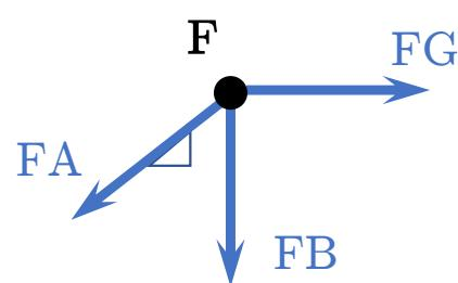
$$\sum F_x = 0 \quad FG - \left[ (-65\sqrt{2}) \frac{3}{\sqrt{18}} \right] = 0 \quad \boxed{FG = -65 \text{ kN}}$$
