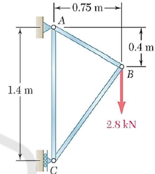
**Example (2):** Using the method of joints, determine the force in each member of the truss shown.
