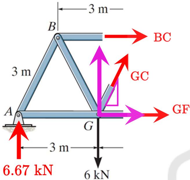
$$\sum M_G = 0 \quad (-BC \times 2.6) + (-6.67 \times 3) = 0 \quad \boxed{BC = -7.69 \text{ kN}}$$
