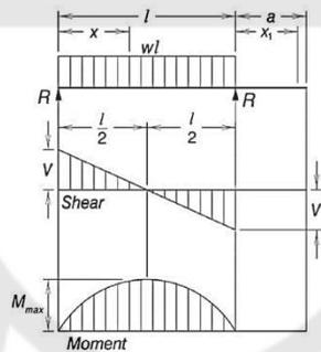
$$\Delta_{max} \text{ (at center)} \dots\dots\dots = \frac{5wl^4}{384EI}$$
