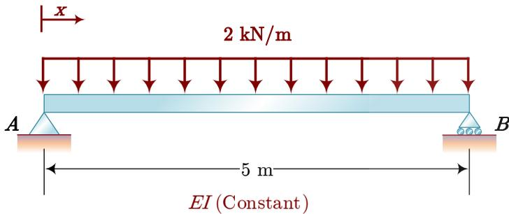
$$w_1 = 2 \frac{\text{kN}}{\text{m}} \times \frac{1 \text{ m}}{1000 \text{ mm}} = 0.002 \frac{\text{kN}}{\text{mm}}$$
