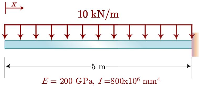
$$w = 10 \frac{\text{kN}}{\text{m}} \times \frac{1 \text{ m}}{1000 \text{ mm}} = 0.01 \frac{\text{kN}}{\text{mm}}$$
