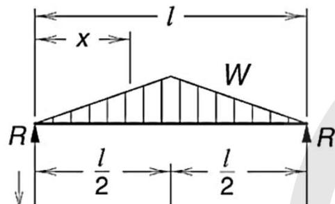
$$W = wl = \left(0.008 \frac{\text{kN}}{\text{mm}}\right)(5000 \text{ mm}) = 40 \text{ kN}$$
