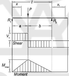
$$\Delta_{max} \left( \text{at } x = \sqrt{\frac{a(a+2b)}{3}} \text{ when } a > b \right) \dots\dots\dots = \frac{Pab(a+2b)\sqrt{3a(a+2b)}}{27EI}$$
