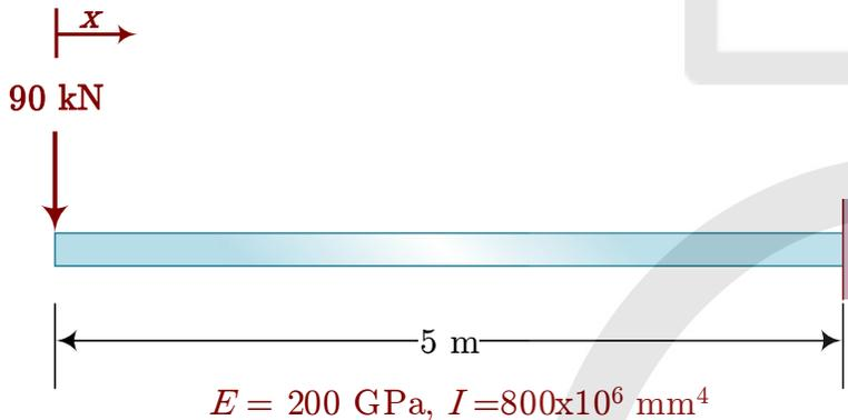
$$\Delta_P = \frac{Pl^3}{3EI} = \frac{(90 \text{ kN})(5000 \text{ mm})^3}{3 \left(200 \frac{\text{kN}}{\text{mm}^2}\right)(800 \times 10^6 \text{ mm}^4)} = 23.43 \text{ mm}$$
